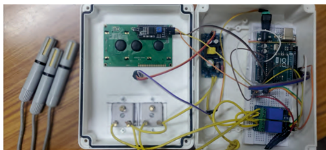
Fig. 7. Microcontroller-based humidity control system with sensors and control circuitry for automatic airflow regulation.
