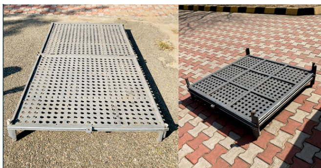
Fig. 6. GFRP perforated drying bed in unfolded and folded configurations for drying operation and easy portability
