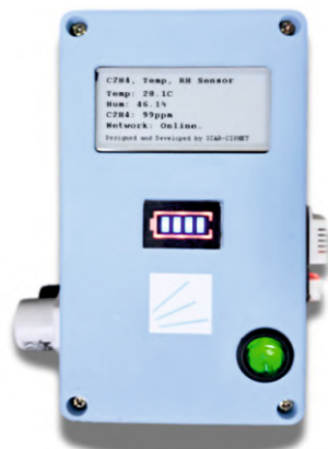
Fig. 15. Sensor-based banana monitoring device; real-time cold storage data
