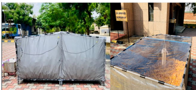
Fig. 5. Field evaluation of the Microcontroller-based maize cob dryer showing the outer structure and transparent roof for solar heat gain.
